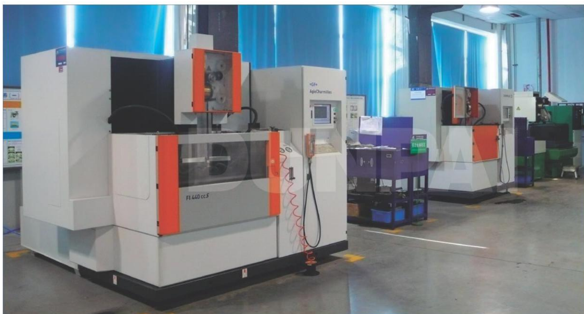
瑞士夏米尔慢走丝线切割机床 / 用于精密加工复合模和级进模 Switzerland CHARMILES Slow Wire Cutting Machine / Used for the manufacture of complex die and the progressive die
