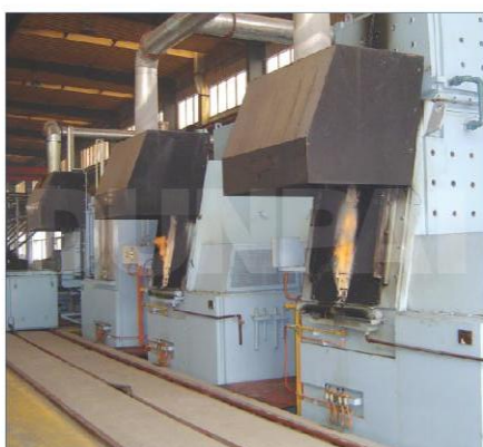
多用热处理炉 / 采用国际先进技术制造的多用炉， 用于销轴、滚子、套筒C-N共渗热处理 Multi-purpose furnace / Multi-purpose furnace which made adopting international advanced technology used for pin, roller & bush carbon-nitriding heat treatment.
