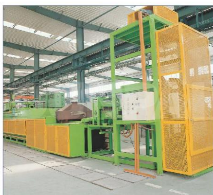
网带炉 / 采用国际先进技术制造的网带炉， 用于滚子、套筒C-N共渗热处理 Mesh belt conveyor furnace / Mesh belt conveyor furnace which made adopting international advanced technology used for roller & bush carbon-nitriding heat treatment.
