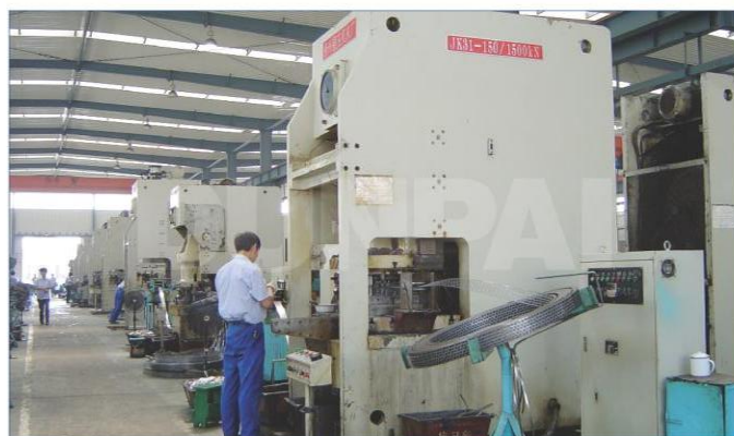
链板自动冲裁 Automatic punching of plates
